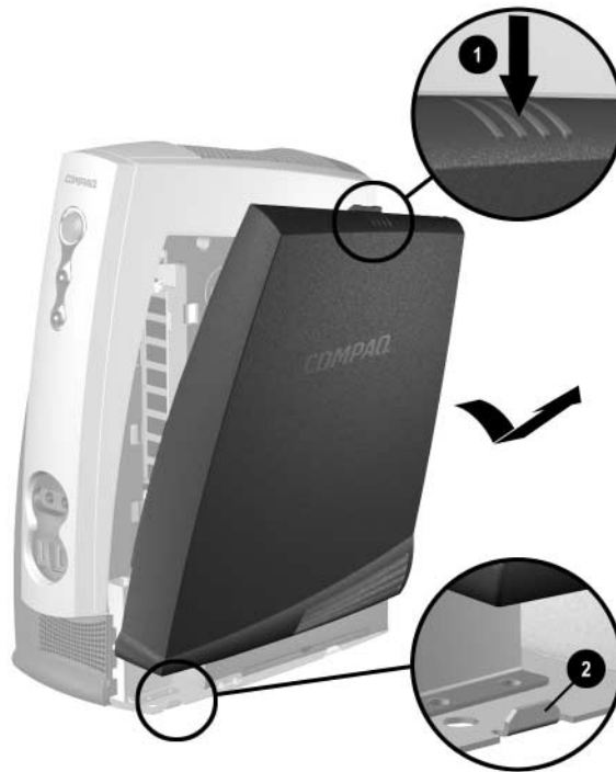
Removing the Right Side Access Panel
